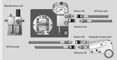
Included in the scope of delivery: hydraulic hoses, 5 m long (DN 6). Accessory: Maintenance unit to increase operational safety and service life of the pneumatic drive. Comes complete with filter, regulator, lubricator and high-pressure hose incl. couplings.
